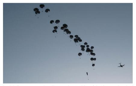
Above: Containerized delivery system bundles are dropped in Afghanistan using the low-cost, low-velocity parachute system. Below: Army riggers prepare bottled water for airdrop in Afghanistan. Since 2001, the airdrop of supplies has been essential to resupplying units in remote locations inaccessible by truck.
