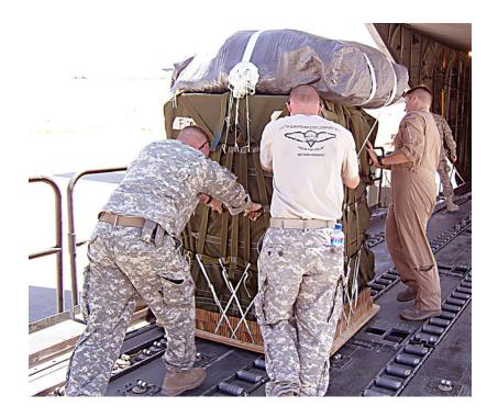
Containerized delivery system (CDS) bundles are loaded onto a C-130 or C-17 aircraft, where riggers will jointly inspect the bundles with Air Force personnel before handing over the airdrop mission.
